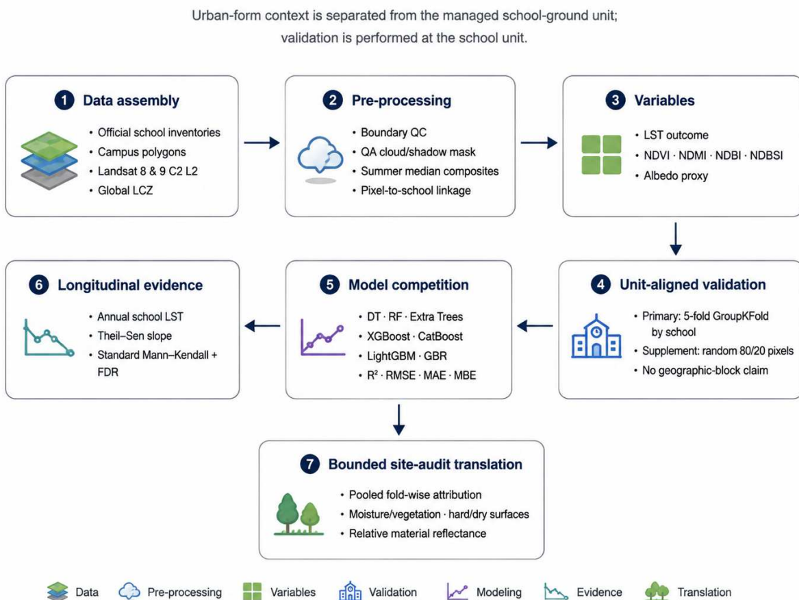
Figure 3. Decision-unit-aligned analytical workflow. LCZ describes surrounding urban-form context, the campus is the managed analytical unit, and primary predictive validation is performed on held-out schools rather than randomly mixed pixels.
