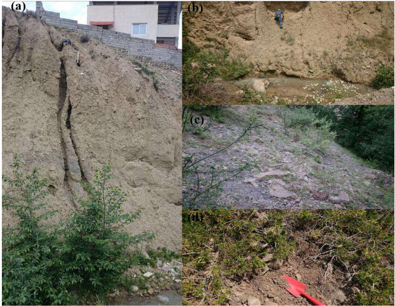
142 Fig. 3 Source sampling. (a) Actively eroding alluvial bank of the Qal unit; (b) sampling an exposed 143 weathered face; (c) bedded exposure in a bedrock unit; (d) composite subsampling with a trowel.
