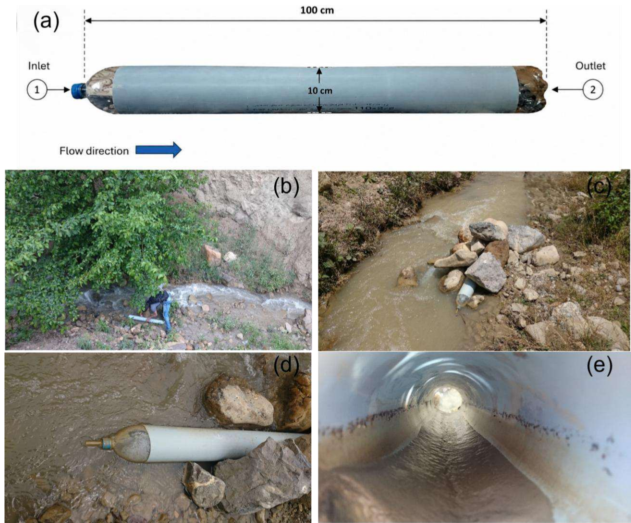
Fig. 2 Time-integrating suspended sediment sampler. (a) Dimensions; water enters at the inlet (1) and leaves at the outlet (2), each a 5 mm aperture, (b) Installation, (c) Sampler anchored in the cross-section, (d) Inlet detail, (e) Sediment retained after a flood.
