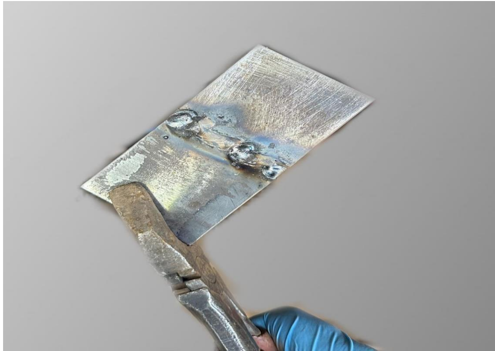
Fig 1. Photograph of the flux-cored arc welded mild steel joint produced using nickel-based filler metal.
