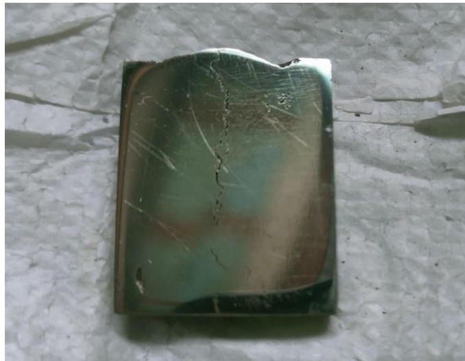
Fig .16. Macro photograph of welded joint showing crack initiation before impact testing.
