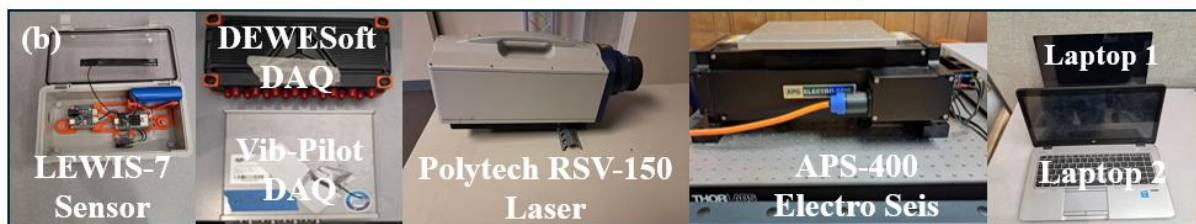
Figure 11: Experiment setup on shaker: (a) overview of sensor setup and (b) the LEWIS 7 sensor, data acquisition device, LDV used in this test, APS-400 Electro Seis shaker, and supporting equipment.
