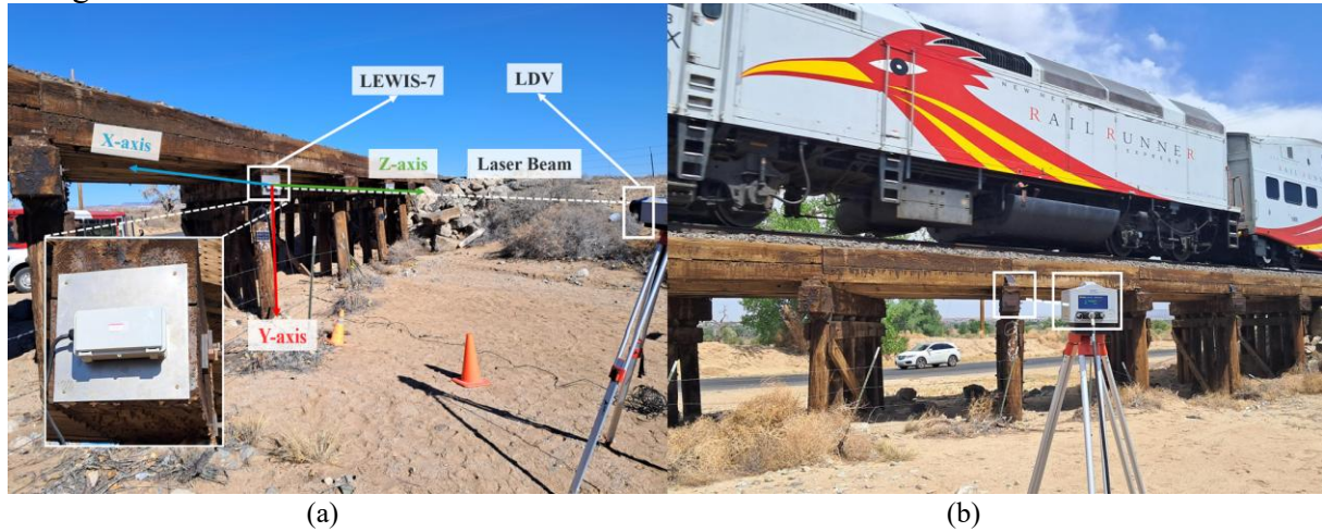
Figure 14: Field validation setup on a timber railroad bridge; (a) laser and sensor relative view from the upstream; (b) railroad crossing event validation monitoring.
