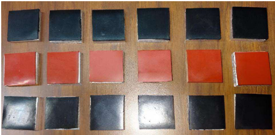
Figure 2. Elastomer samples evaluated as coating materials for the AFP compaction roller.
