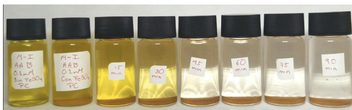
Fig. 7 Visual change in the color of the AO solution during ferrous-species-assisted corona plasma treatment, from the initial condition to 90 min of treatment.
