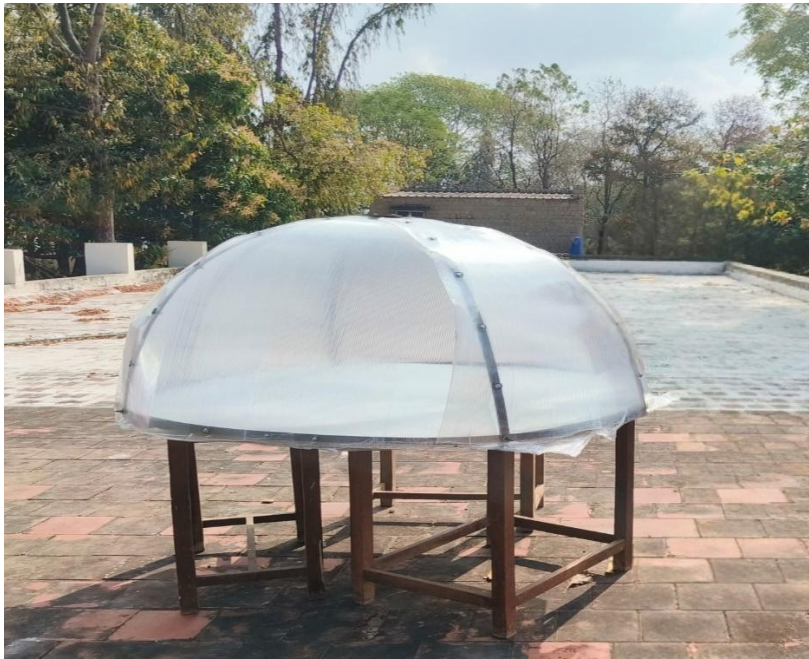
Figure 1. Experimental hemispherical solar greenhouse used for outdoor thermal performance evaluation under natural solar radiation
