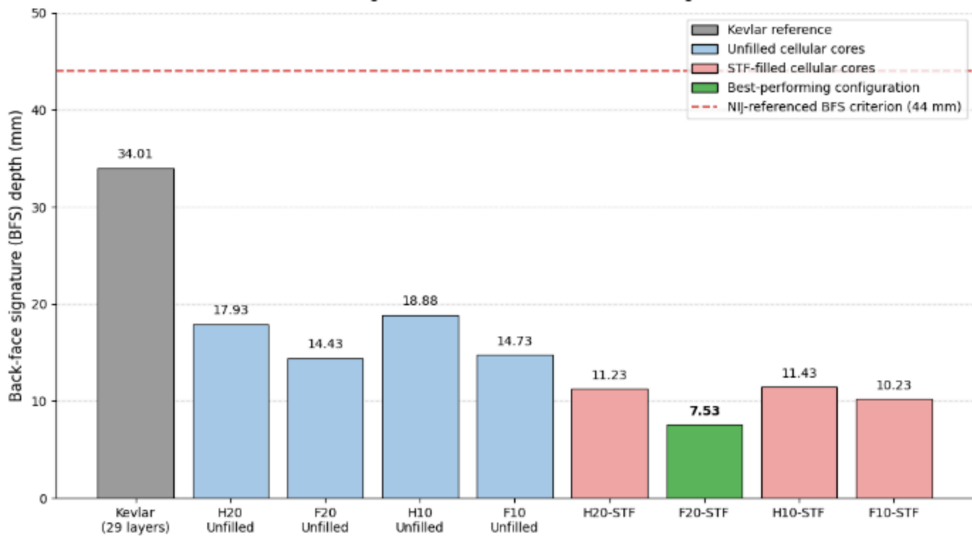
Figure 7 Back-face signature depths of the Kevlar-only reference, unfilled cellular-core panels, and STF-filled composite panels after ballistic impact testing.
