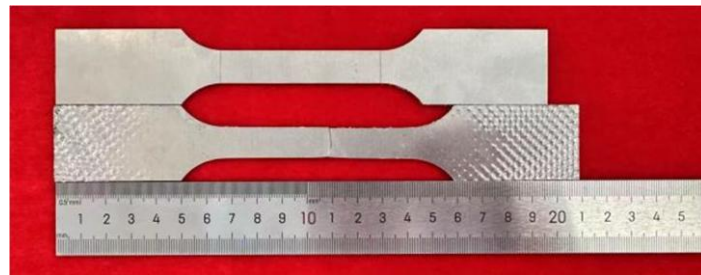
Fig. 5 Comparative image of the 2A12-T4 aluminum alloy specimen before and after tensile testing
