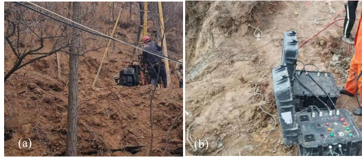
Fig. 1 Field evidence used to constrain the model: (a) borehole drilling on the natural slope, (b) in-hole wave-velocity testing
