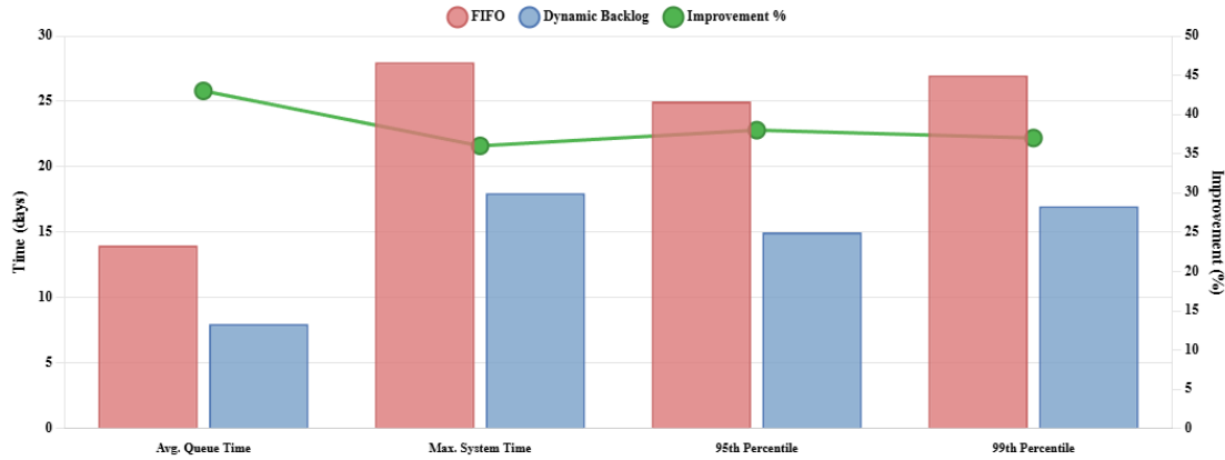
Figure 4: Comparison of temporal metrics between FIFO (red) and Dynamic Backlog (blue); green line indicates improvement percentages (37–43%). Consistence ( \sigma = 2.8\% ); Welch: p -value < 0.001 , Cohen's d = 1.84 .
