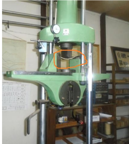
Fig.3 Universal Testing Machine (UTM) setup in the mechanical testing laboratory showing the three-point bending fixture and loaded composite specimen.
