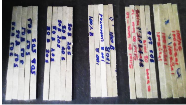
Fig.1 Prepared test specimens for flexural testing showing different fiber composition ratios (100S, 100B, 80S20B, 50S50B, 20S80B).
