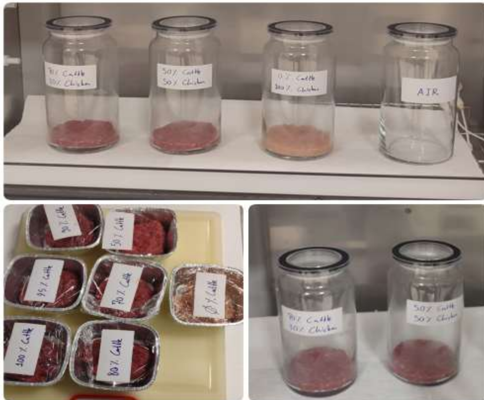
Figure 4. Meat mixtures prepared at different cattle-to-chicken ratios used for sensor measurements, and the laboratory environment in which the experiments were conducted.
