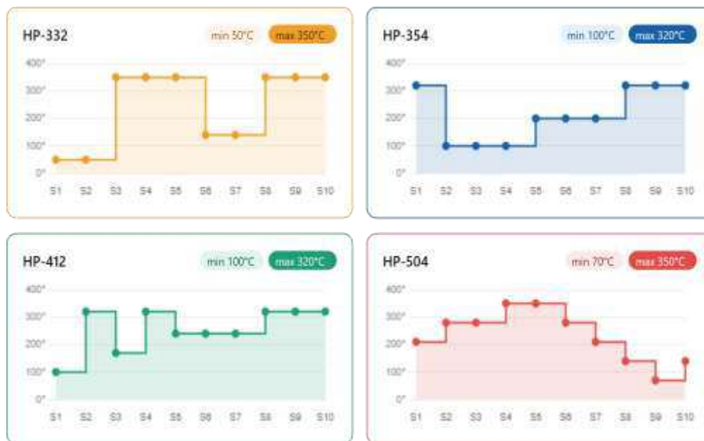
Figure 3. Temperature modulation profiles applied to the BME688 sensor array in this study (HP-332, HP-354, HP-412, and HP-504).
