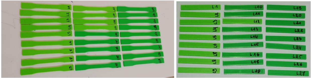
Fig. 1. PLA printed samples images by FDM printer (a) tensile test (b) three-point flexural test.
