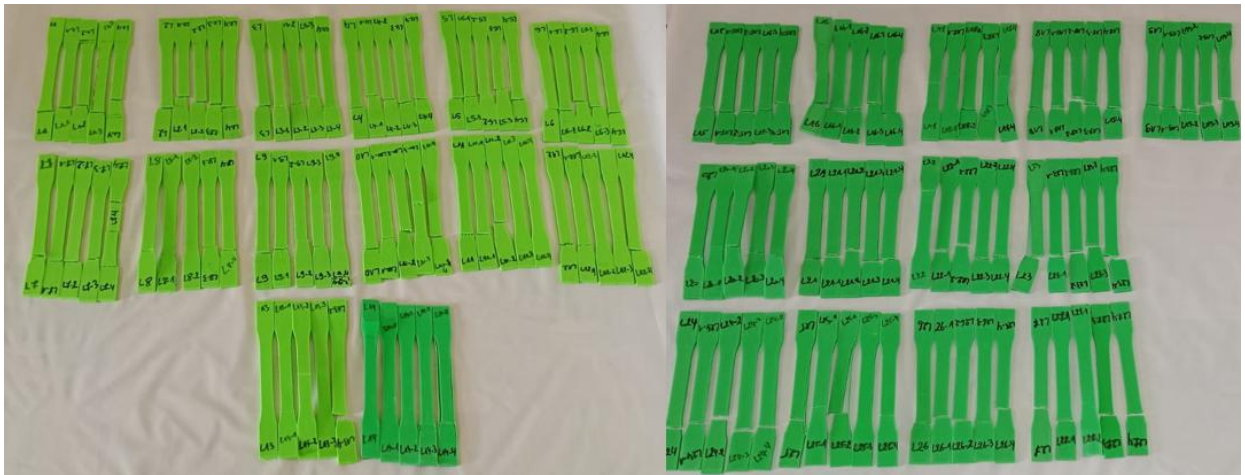
Fig. 4. Image of PLA samples after tensile testing.
