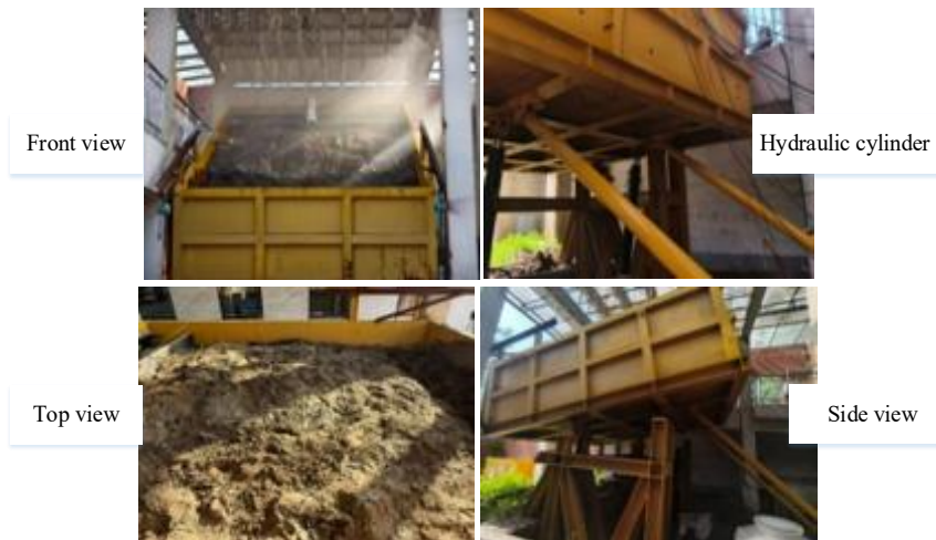
Figure 2. Details of the landslide simulation test chamber.
