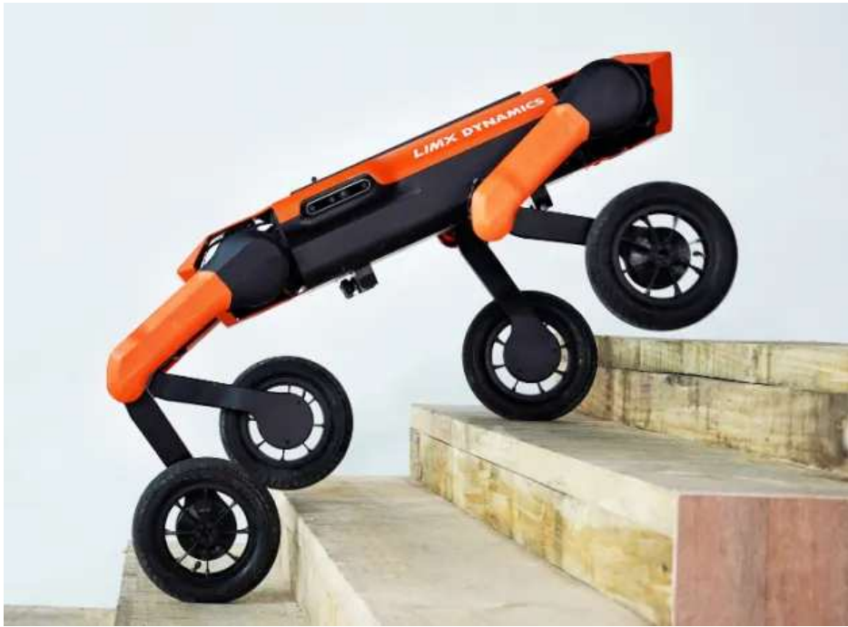
Fig. 1: The W1 wheeled quadrupedal robot (LimX Dynamics) used as the hardware platform. The system features 16 actuated DoFs (12 leg joints and 4 active wheels).
