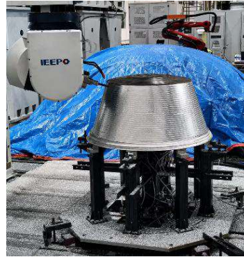
(b) Milling experiment of thin-walled conical shell
