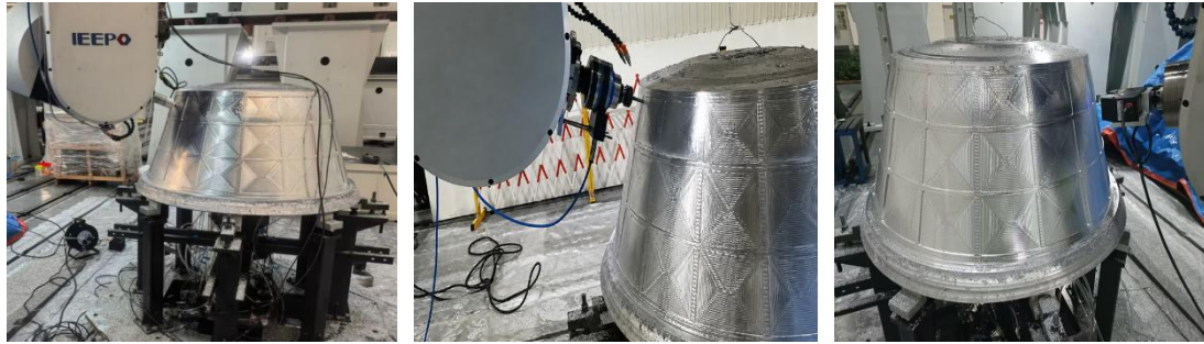
(a) Electromagnetic ultrasonic wall thickness on-machine scanning (b) Milling force on-line monitoring (c) Line laser profile on-machine scanning
