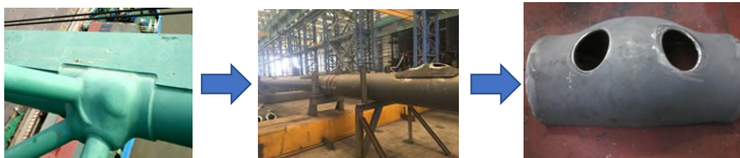
Fig. 3 Morphological evolution process of bulge-formed joint surface
