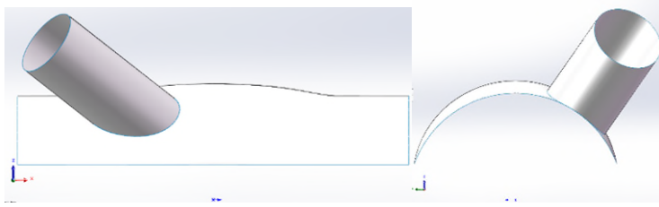
Fig. 23 Optimized bulge-formed joint
