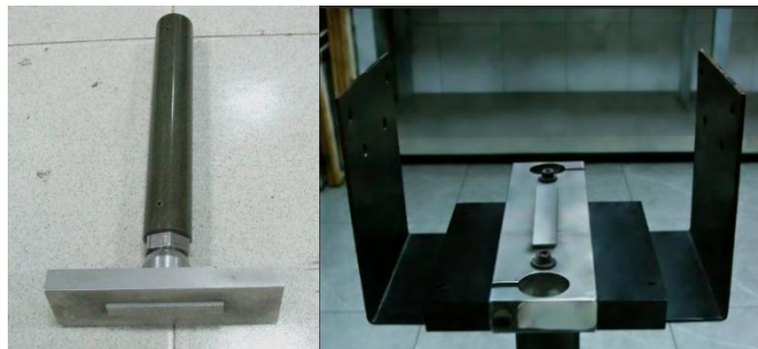
Figure 6. Improved spherical-hinge IDT test fixture.
