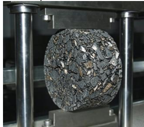
Figure 5. Double-limiting cylinder IDT test fixture.
