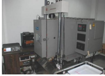
Figure 4. MTS 810 electro-hydraulic servo material testing system.
