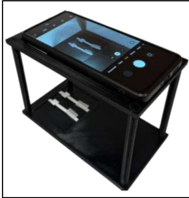
Figure S3. Custom 3D-printed smartphone holder used to ensure reproducible imaging conditions during LFA analysis. The device consists of an upper platform supporting the smartphone at a fixed height of 12 cm and a lower compartment designed to accommodate the LFA strips. This configuration ensures a constant imaging geometry and was maintained in the same position for all acquisitions to guarantee consistent photographic conditions.
