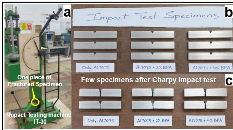
Fig.8. (a) Impact Testing machine (b) Impact test Specimens (c) few specimens after testing
