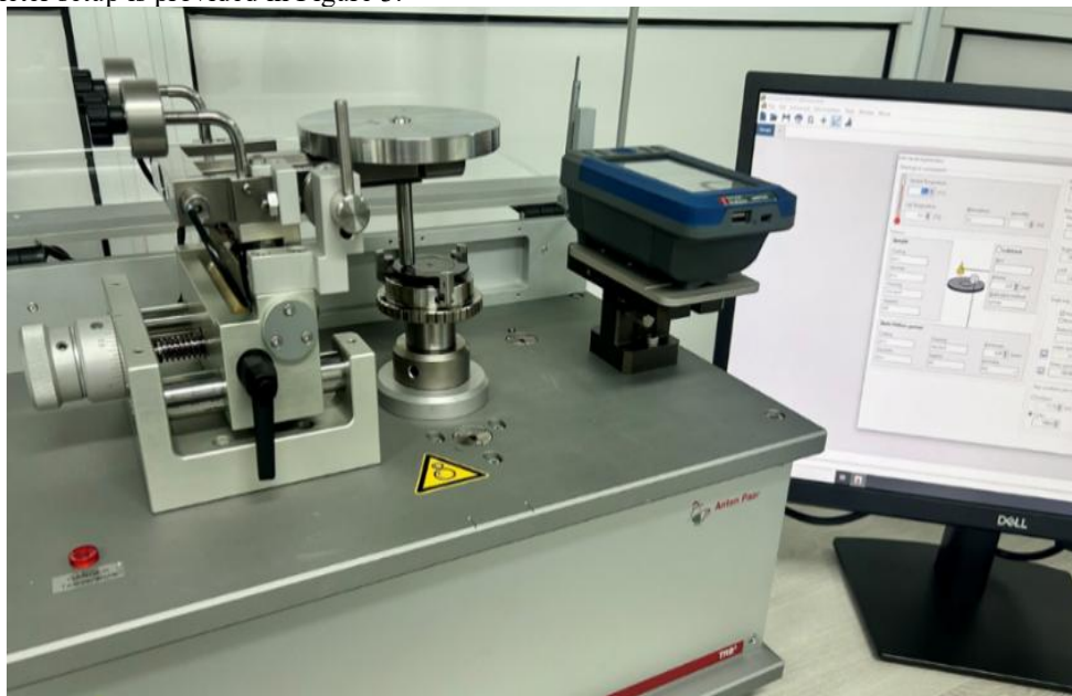
Figure 2. Anton Paar TRB 3 pin-on-disc tribometer: (a) instrument overview; (b) close-up of the contact zone with composite disc (lower) and steel ball holder (upper).
