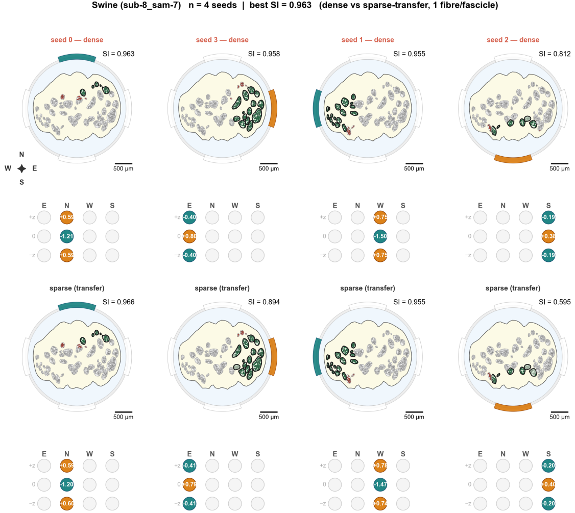
Figure S39: Specimen swine sub-8_sam-7 . All target-cluster seeds for this nerve, ordered left-to-right by achievable selectivity index SI. Each seed shows the nerve cross-section (top) with fibers colored by post-optimization recruitment (target fired / target silent / off-target fired / off-target silent) and the peripheral target-fascicle cluster outlined, above the optimized 12-contact cuff pattern (bottom; cathode blue, anode orange, inactive white, marker size \propto |I_k| , over four angular columns \times three axial rows).
