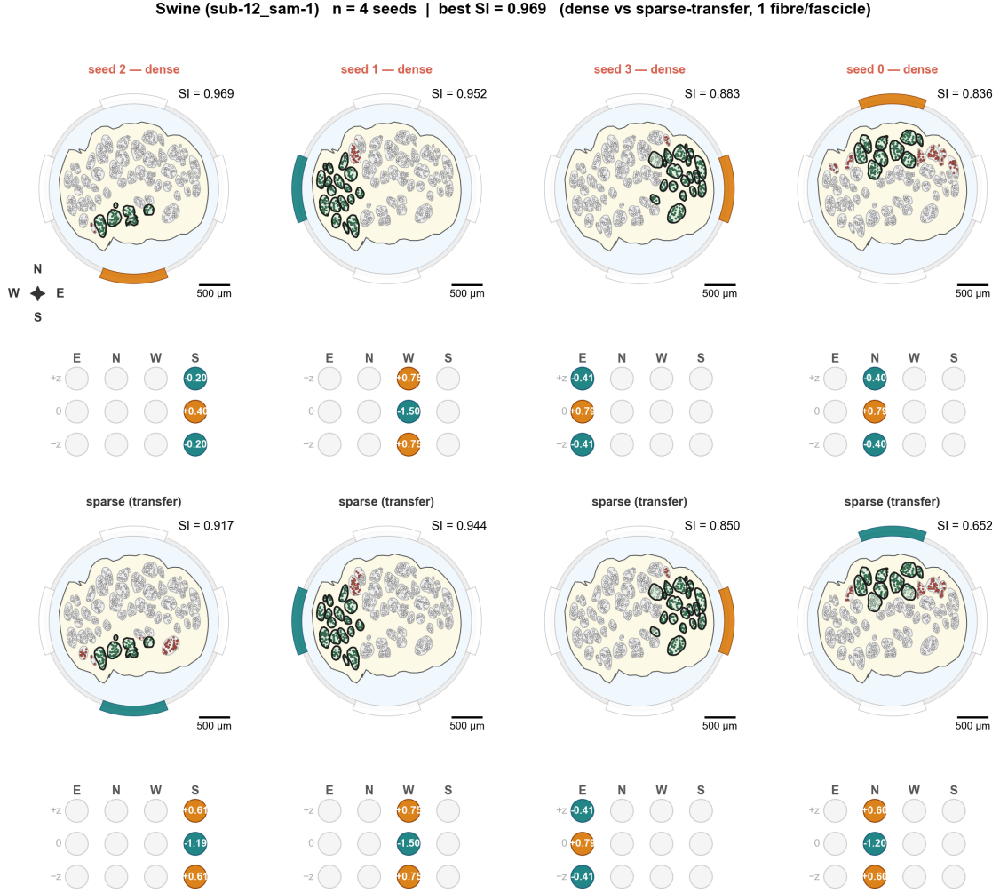
Figure S44: Specimen swine sub-12_sam-1 . All target-cluster seeds for this nerve, ordered left-to-right by achievable selectivity index SI. Each seed shows the nerve cross-section (top) with fibers colored by post-optimization recruitment (target fired / target silent / off-target fired / off-target silent) and the peripheral target-fascicle cluster outlined, above the optimized 12-contact cuff pattern (bottom; cathode blue, anode orange, inactive white, marker size \propto |I_k| , over four angular columns \times three axial rows).
