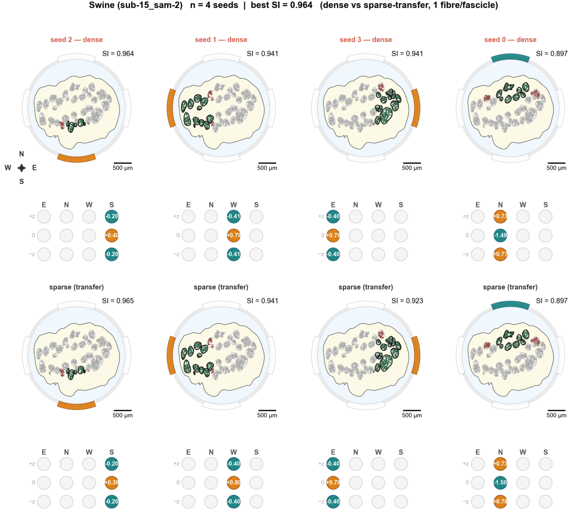
Figure S50: Specimen swine sub-15_sam-2 . All target-cluster seeds for this nerve, ordered left-to-right by achievable selectivity index SI. Each seed shows the nerve cross-section (top) with fibers colored by post-optimization recruitment (target fired / target silent / off-target fired / off-target silent) and the peripheral target-fascicle cluster outlined, above the optimized 12-contact cuff pattern (bottom; cathode blue, anode orange, inactive white, marker size \propto |I_k| , over four angular columns \times three axial rows).
