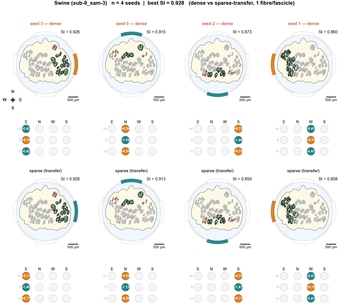
Figure S40: Specimen swine sub-9_sam-3 . All target-cluster seeds for this nerve, ordered left-to-right by achievable selectivity index SI. Each seed shows the nerve cross-section (top) with fibers colored by post-optimization recruitment (target fired / target silent / off-target fired / off-target silent) and the peripheral target-fascicle cluster outlined, above the optimized 12-contact cuff pattern (bottom; cathode blue, anode orange, inactive white, marker size \propto |I_k| , over four angular columns \times three axial rows).
