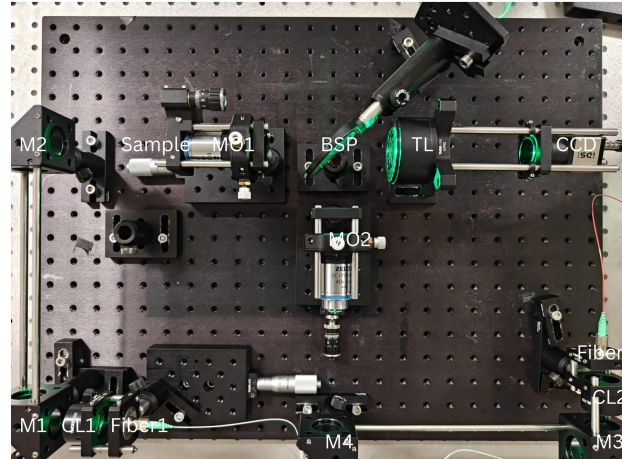
Figure 2: Schematic depicting the second digital holographic microscope imaging system.
