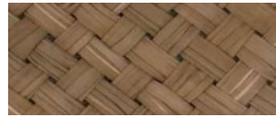
Fig. 2. Over-Two Weave Pattern
