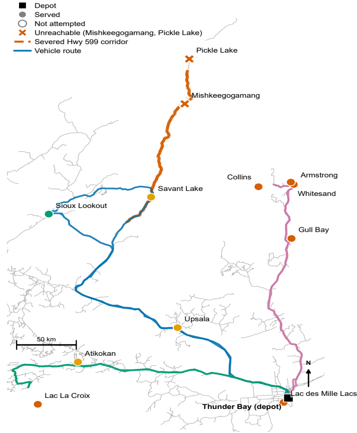
Figure S5. Executed relief plan for the real twelve-community instance under realistic parameters, showing depot routes from Thunder Bay. Communities are marked as served, unattempted, or unreachable. Mishkeegogamang and Pickle Lake are unattempted due to Highway 599 closure from day 3, resulting in identical risk-aware and risk-blind routes.
