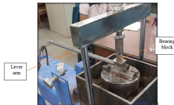
Figure 7. Assembly of the TDST apparatus: (a) bearing block and lever-arm connection; (b) load-cell and winch coupling
