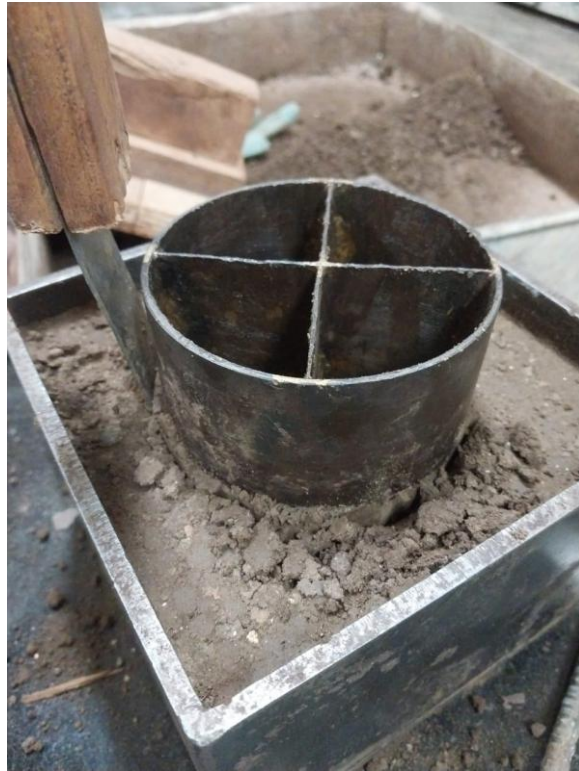
Figure 4. Details of the vane (90 mm / 60 mm diameter interchangeable vanes)
