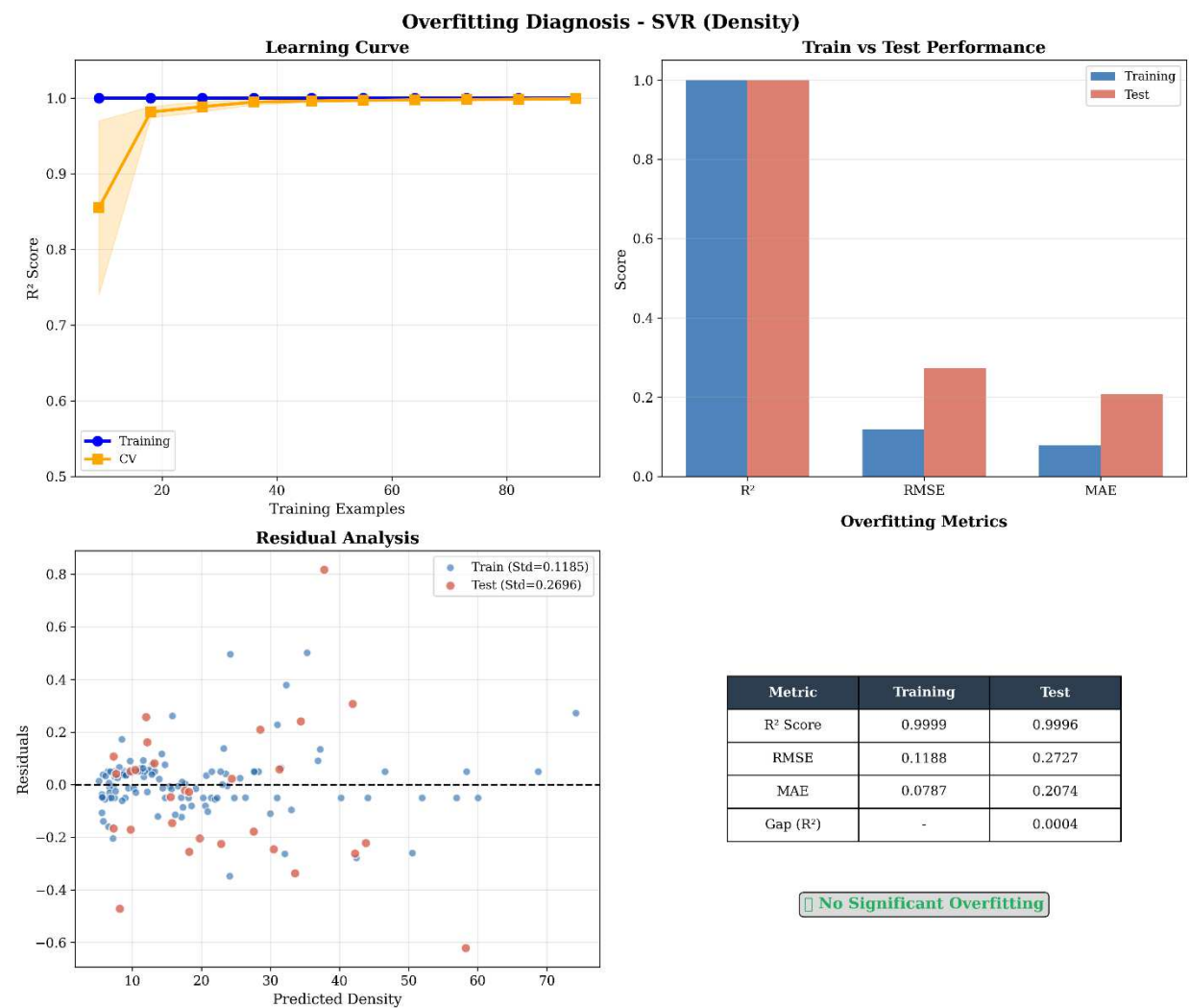
Fig. 5. Overfitting diagnosis for the SVR-RBF model applied to density prediction: learning curve, training vs. test performance comparison, residual analysis, and performance gap summary.
