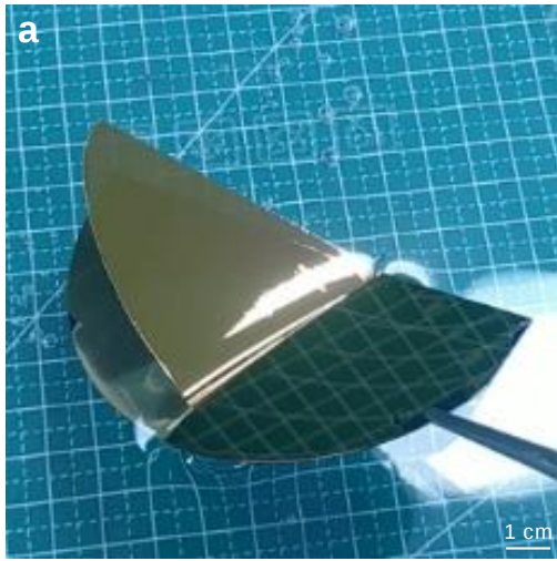
Supplementary Fig. 5 | Exfoliation of the Au film. a , Photograph of the exfoliation process for a wafer-scale Au film. b , Photograph of the free-floating Au film on water after exfoliation. Inset: the initial Au film on the \text{SiO}_x/\text{Si} substrate prior to exfoliation.
