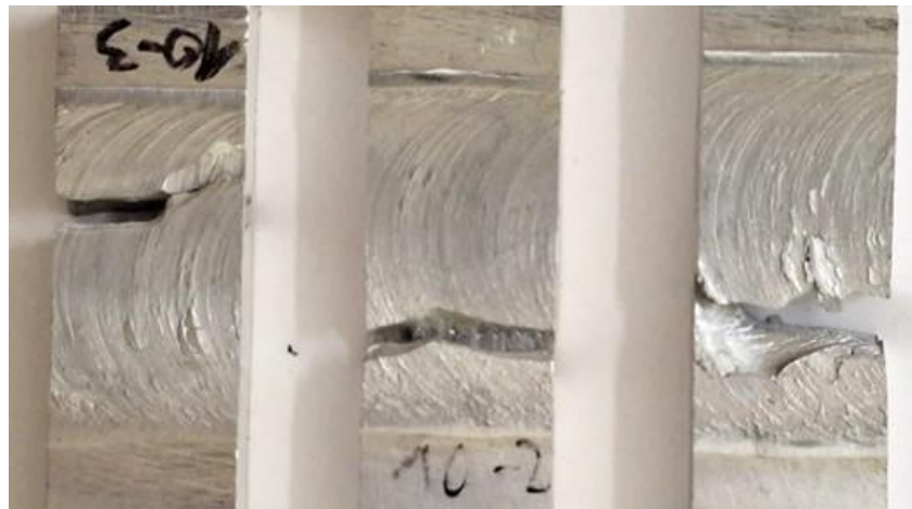
Fig. 11. Fracture locations of FSW joints produced in air at tool rotational speeds of 1000 rpm after static tensile testing.
