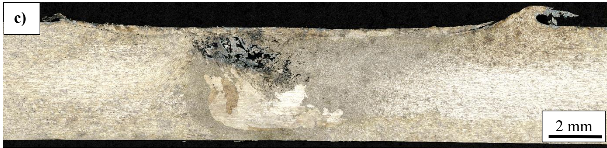
Fig. 2. Macrostructural images of selected samples: 600+HT (a), 1000+HT (b), 1400+HT (c).
