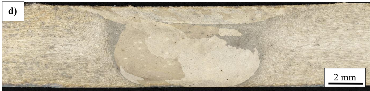
Fig. 4. Macrostructural images of selected samples: Air+HT (a), OH-70+HT (b), Water+HT (c), 10%CF+HT (d).
