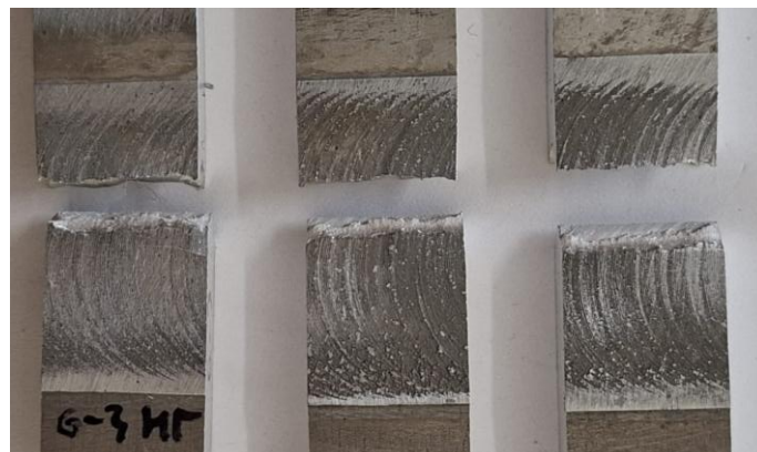
Fig. 13. Fracture location of the 600+HT specimen after static tensile testing.
