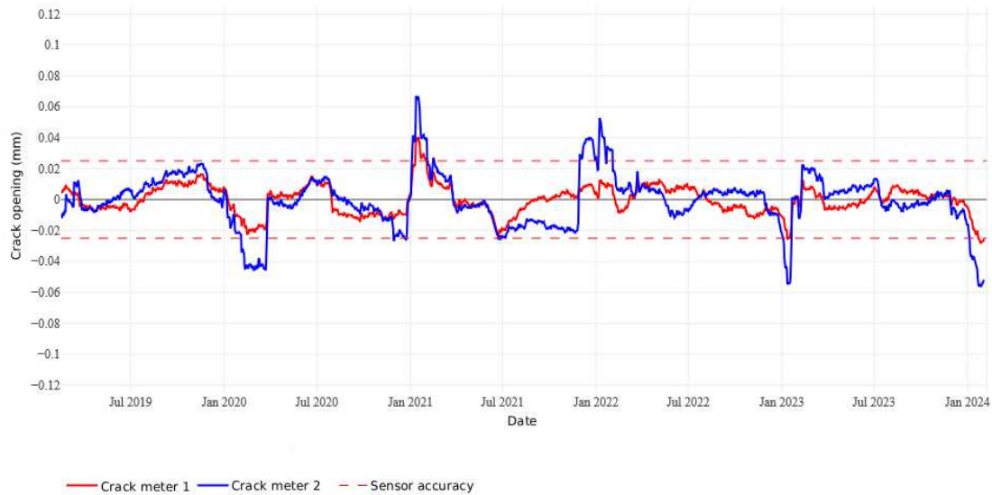
Fig. 23 Isolated stationary residual components \epsilon(t) for Crackmeter 1 and Crackmeter 2.
