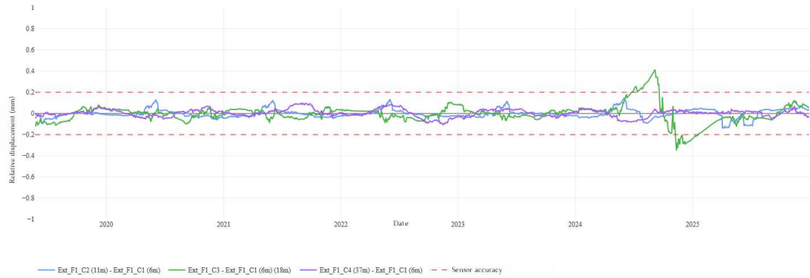
Fig. 19 Relative inter-anchor differential displacement derived from stationary residual components for the "Rue" extensometer (Borehole F1).
