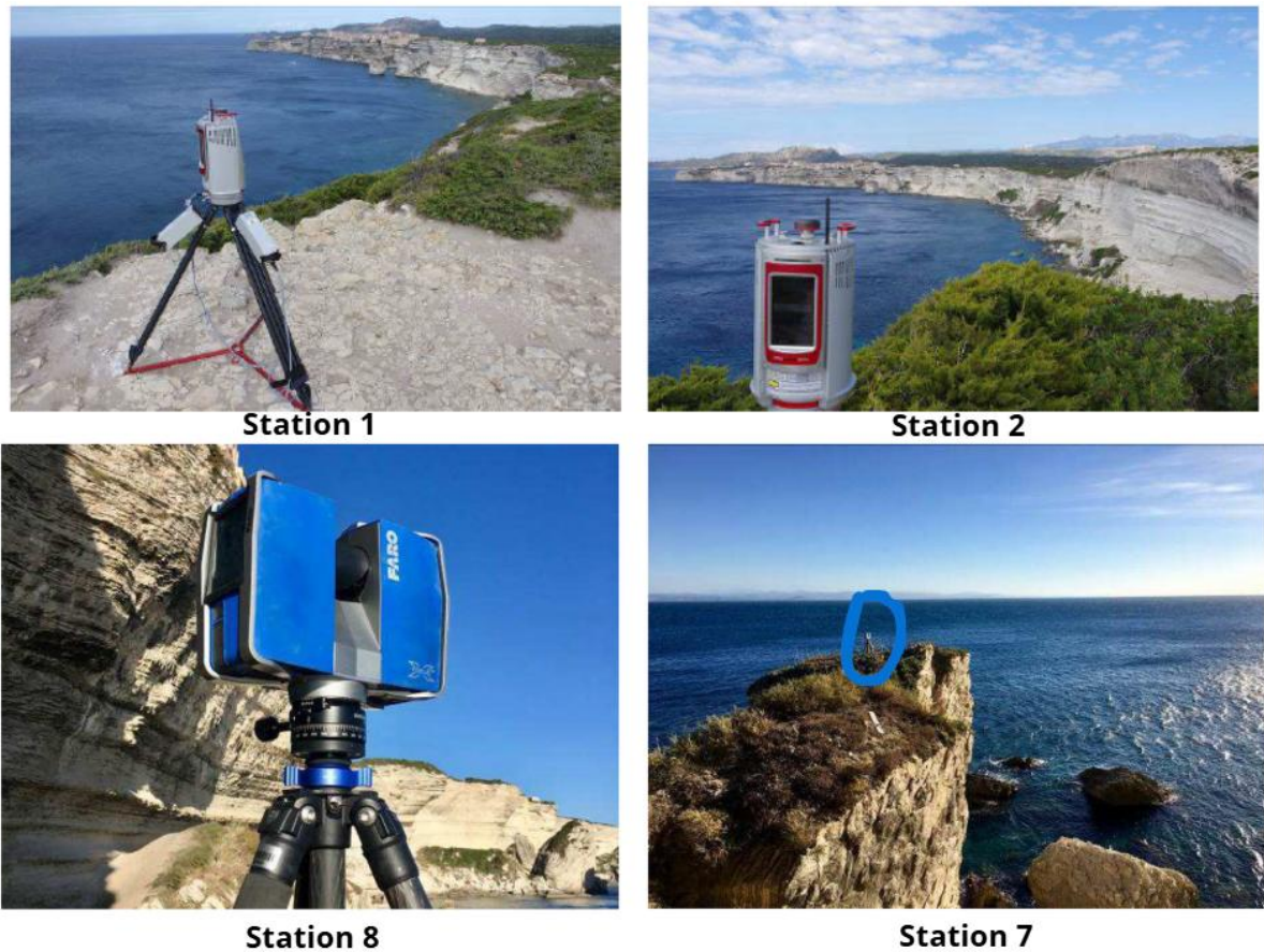
Fig. 3 : Terrestrial Laser Scanner (TLS) stations used for monitoring the cliff profile: Station 1 and Station 2 set up on the top of the cliff, Station 8 installed at the base of the cliff, and Station 7 positioned on the headland overlooking the study area.
