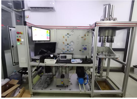
Fig. 1. Top 50 HT multi-field coupled rock rheometer
