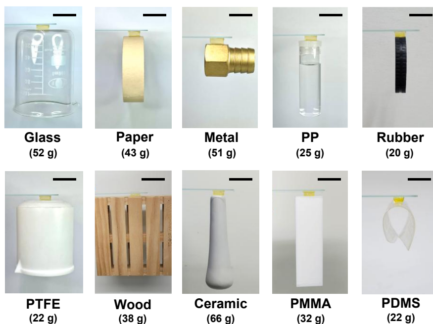
Supplementary Fig. 11 Photographs of the PIL/IL ionogel with excellent adhesion to various representative substrates. The top side of Ionogel-75 is adhered to a glass slide, and the other side is adhered to the surfaces of various materials. Then, the glass slide lifted each sample with the ionogel, and remained firmly holding the sample for more than 1 hour without any obvious peeling gaps. The results indicated that the as-prepared ionogel had excellent adhesion properties for various substrates. Scale bar, 20 mm.
