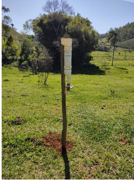
Fig. 2 Precipitation monitoring equipment. The image shows the custom-built PVC rain gauge (150 mm diameter) installed 1.50 m above ground level. The apparatus was positioned in an open area within the study site to ensure accurate rainfall depth ( P ) measurements by avoiding canopy interception
