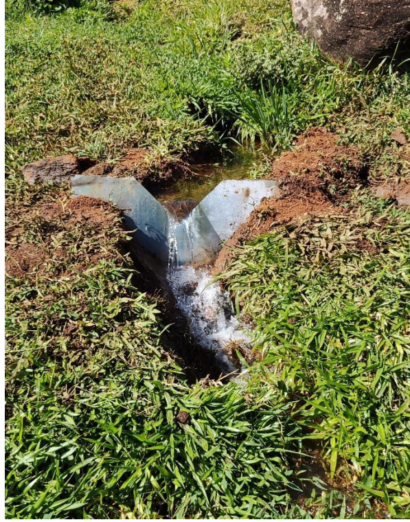
Fig. 4 Streamflow quantification using the weir method. The image illustrates a triangular V-notch weir installed in the stream channel for discharge ( Q ) monitoring. This instrumentation allowed for continuous flow assessment during the pre-mining phase, providing a baseline for the evaluated micro-watersheds.
