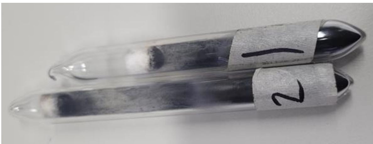
Supplementary Figure 31 A photo of samples in close ampoules for QENS measurement
