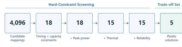
Fig. 1. Feasible-domain contraction in the canonical rerun. Hard constraints reduce 4096 candidate mappings to 15 feasible mappings; Pareto screening retains five.
