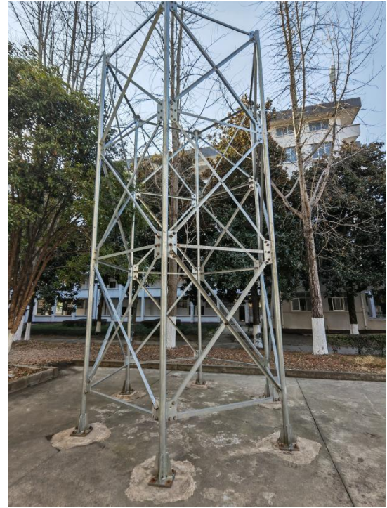
(b) Experimental model of a hexagonal-section steel tubular truss tower
