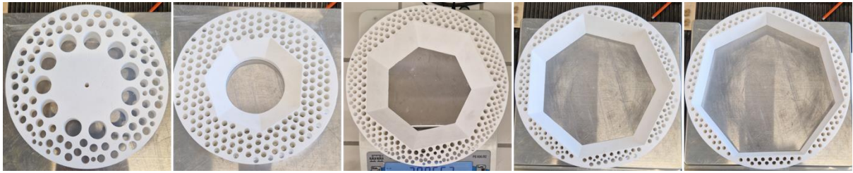
Figure S3: Photographs of the five rings comprising the back ZY3 insulation part after drilling.
