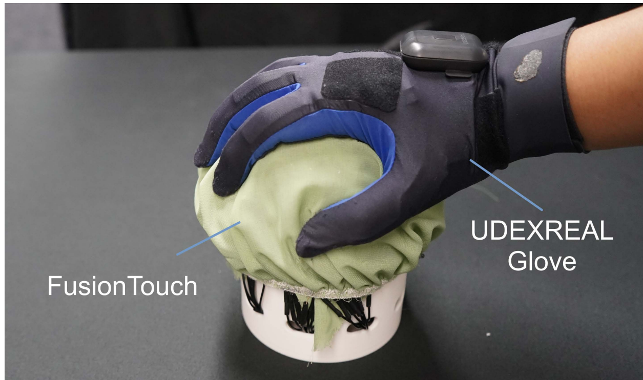
Fig. S21. Hand-gesture data acquisition setup using the UDEXREAL data glove. The image shows the experimental setup used to collect hand-joint motion data during interaction with FusionTouch. A participant wore a UDEXREAL data glove while grasping and deforming the FusionTouch sensing surface. The data glove recorded the joint states of the fingers during different hand gestures, while FusionTouch simultaneously captured contact-induced tactile responses from the soft sensing interface. This setup enabled synchronized acquisition of hand-gesture information and tactile deformation data, providing paired data for analyzing the relationship between finger joint configurations and tactile interaction patterns.
