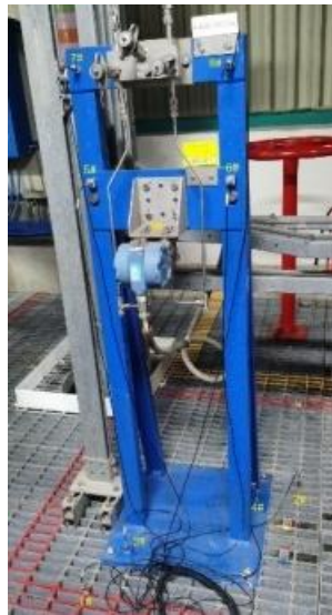
Figure 2 Arrangement of Vibration Measurement Points on Flow Meter Bracket
