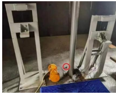
Figure 10 Arrangement of Test Prototypes and Excitation Source
