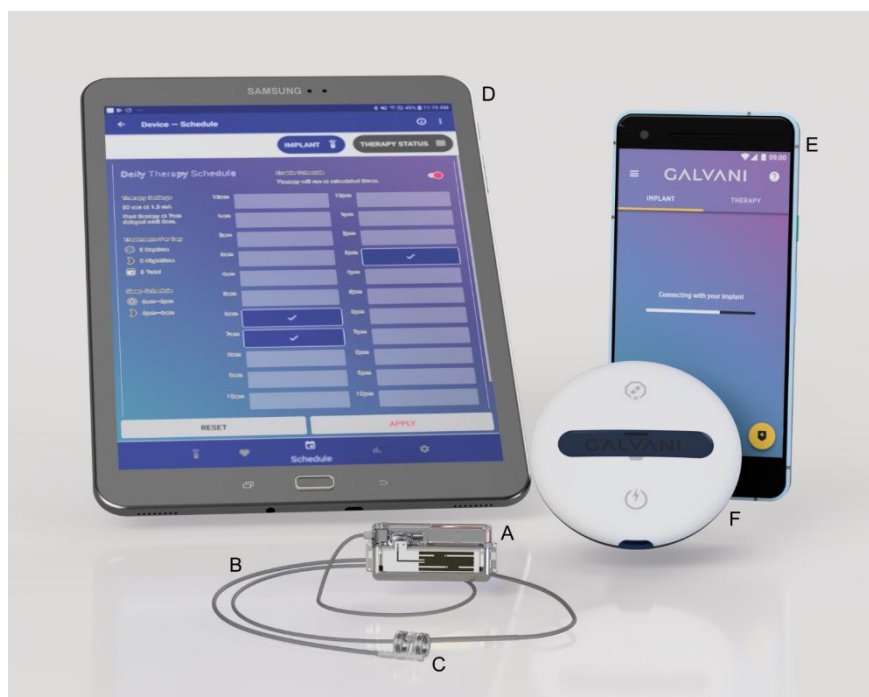
Figure 1: Galvani System. A: IPG, B: Lead, C: Cuff Electrode, D: Clinician Programmer (CP), E: Patient Remote (PR), F: IPG Charger
