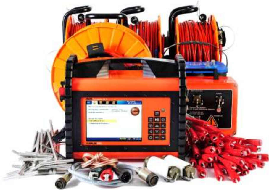
Fig. 7 Geophysical instrumentation used for ground resistivity measurement [29]
