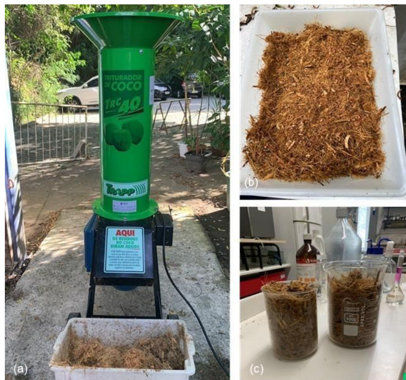
Fig 4 Coconut Crushing (a), Coconut Waste Sample after crushing (b) and (c)
