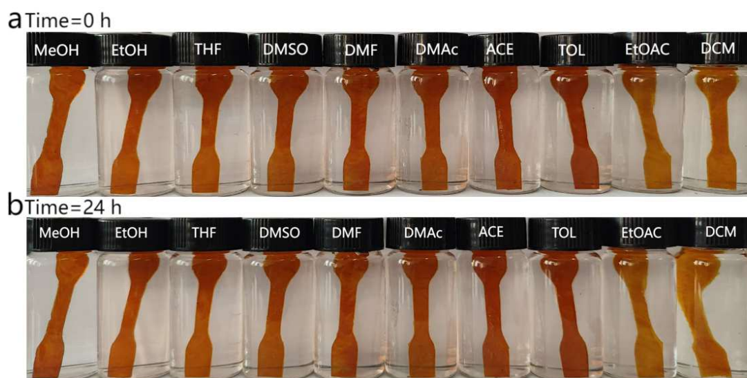
Figure 9. TBD-3 immersed in different solvents at room temperature for 0 hours (a) and 24 hours (b).
