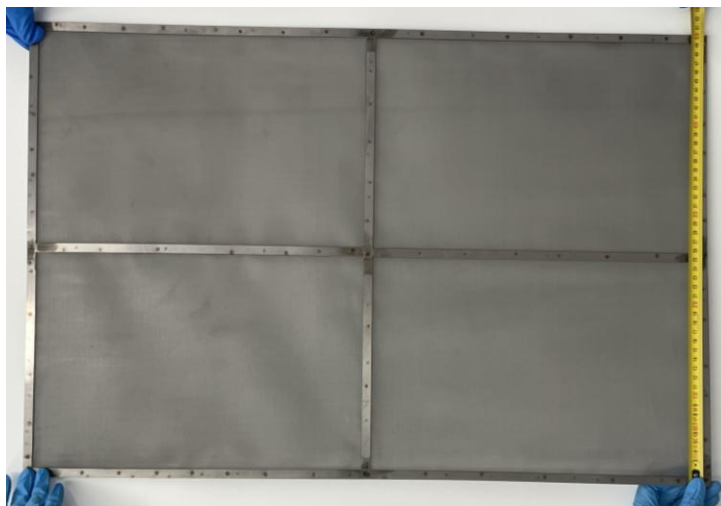
Supplementary Figure S68. Photograph of a large-scale P-Co 1 O 5 monolithic electrode (75 cm × 50 cm) before annealing treatment.
