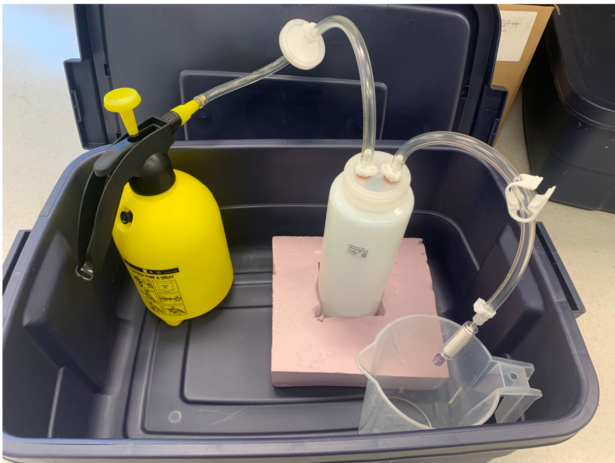
Figure S1. Photograph of filtration set-up for field processing of water samples onto a Sterivex filter.
