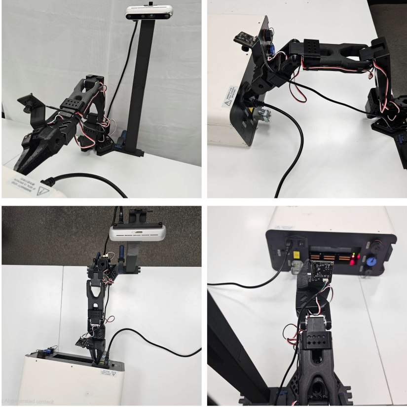
Figure 1: Experimental setup showing the SO101 6-DOF robotic arm with dual-camera vision system. The overhead Intel RealSense D455 camera provides global scene understanding, while the wrist-mounted camera enables close-up manipulation feedback. The system operates in a tabletop workspace with consumer-grade GPU hardware (RTX 4060 8GB), demonstrating the feasibility of deploying large-scale VLA models on affordable platforms.
