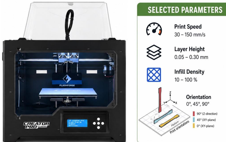
Figure 2 3D printer FDM and selected parameters to be optimized by Taguchi method
