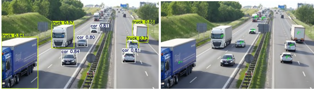
Figure 3. Detection vs. KF-Based Tracking with ID Preservation in Simulated Real-Time Frames
