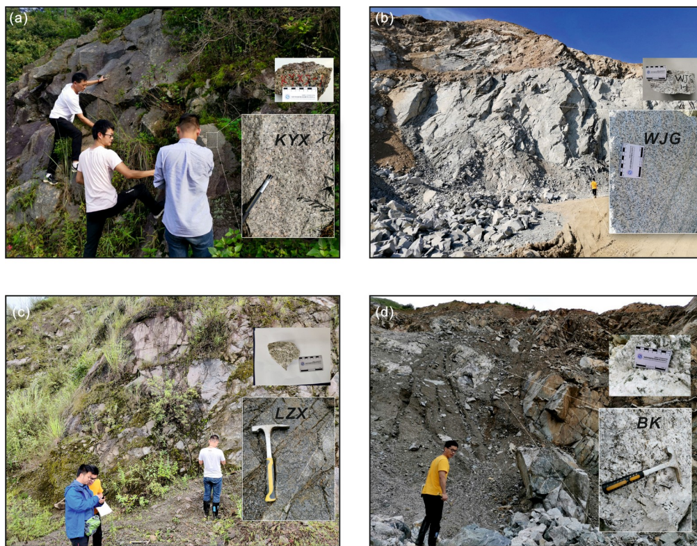
Figure S2. Field photographs, hand specimens, and representative rock textures of the studied plutons in the Mianning–Xichang area. (a) KYX quartz syenite; (b) WJG granite; (c) LZX pluton sample; (d) BK granite.
